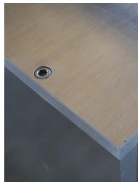
Fig 10: Showing the recessed allan head screws, and the precision of the boxes' fabrication by the company, Lippincott, in North Haven, Connecticut. Photo. B. Ely, 2008.
